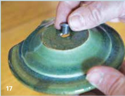
17 Insert the short screw from the plunger assembly into the hole from the top of the lid.
