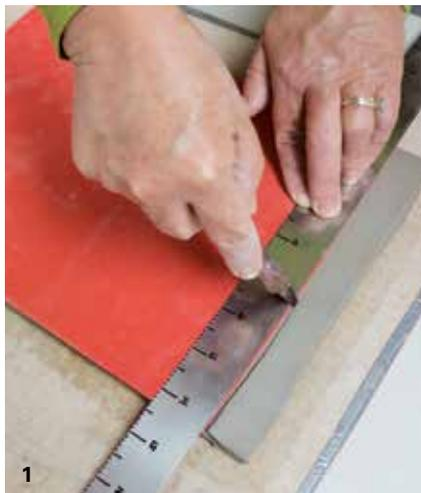
1 When cutting the template on the short sides, hold the knife at an angle to create an even bevel join and a smooth seam.
