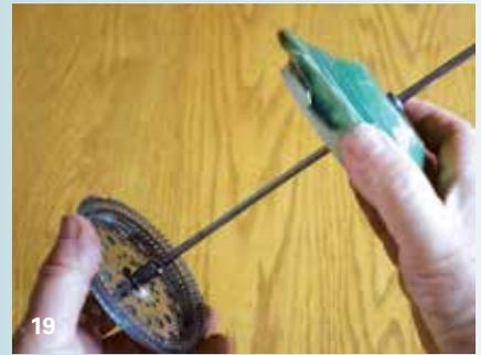
19 Insert the plunger assembly through the bottom of the lid, then add a knob to hold it in place.
